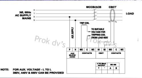
DIGITAL MICROCONTROLLER / MICROPROCESSOR BASED EARTH LEAKAGE RELAY(ELR) -HIERARCHY (Time & Current sensitivity)
