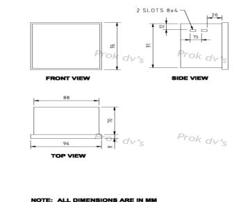
NOTE: ALL DIMENSIONS ARE IN MM TOLERANCE:-±1MM
